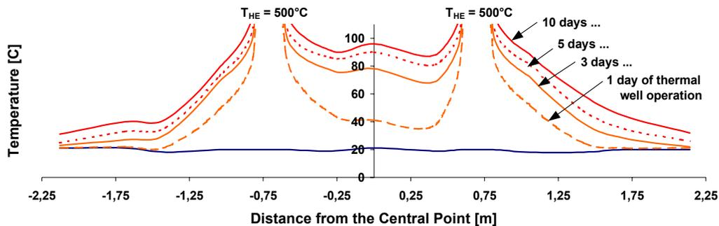
**FIGURE 4: Temporal subsurface temperature development in the diagonal section of the container in the middle of the layer of low permeability.**
