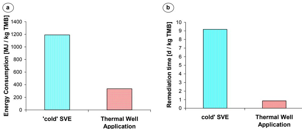
**FIGURE 5: Comparison between ‘cold’ SVE and SVE with additional thermal well application: a) Energy Consumption per kg TMB-extraction, b) remediation time per kg TMB Extraction.**
