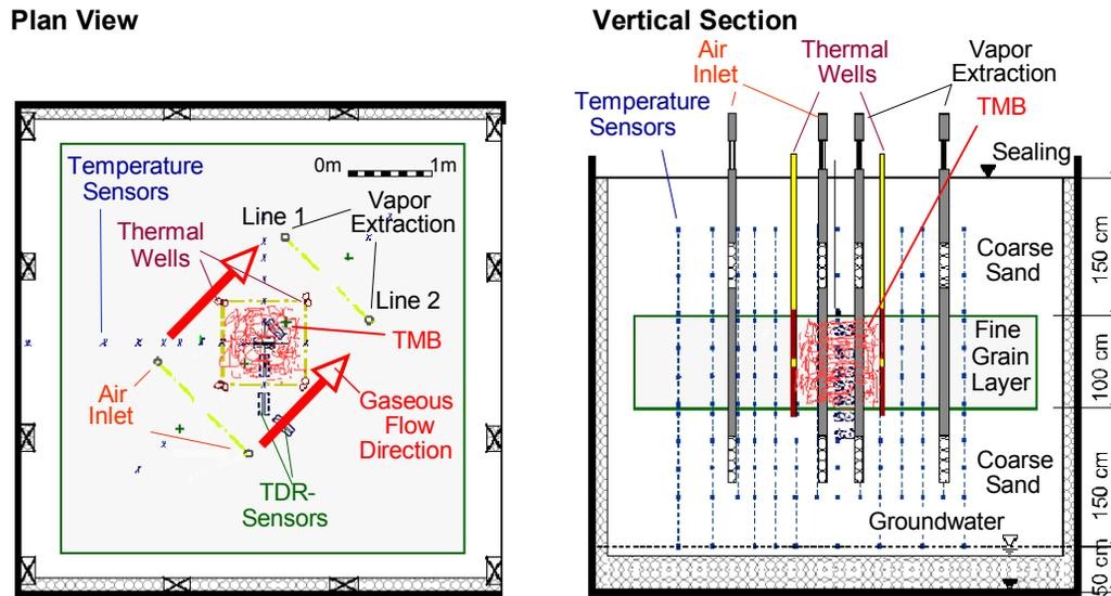
FIGURE 2: Plan view and vertical section of the VEGAS large-scale container.
