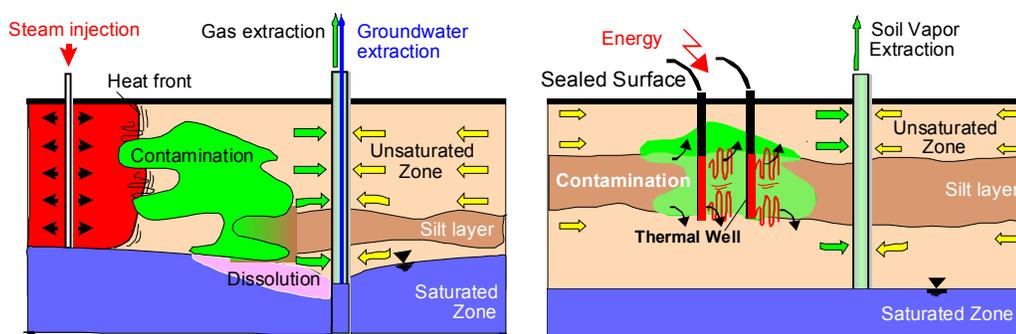
FIGURE 1: Principle of steam injection (left) and thermal wells (right).
