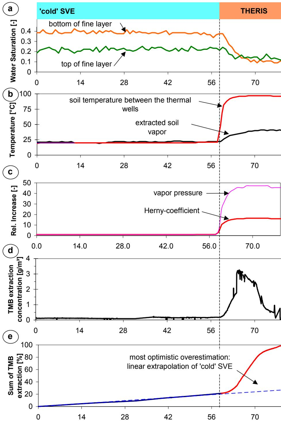
**FIGURE 3:** Development over time of: a) water saturation, b) temperatures, c) relative increase of vapor transfer processes, d) TMB extraction concentration, e) sum curve of extracted TMB
