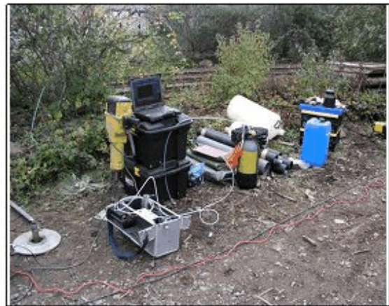
Abb. 9: Metalloxid-Sensorsystem VEGAS (links: Sensorkoffer, rechts: Feldeinsatz)
