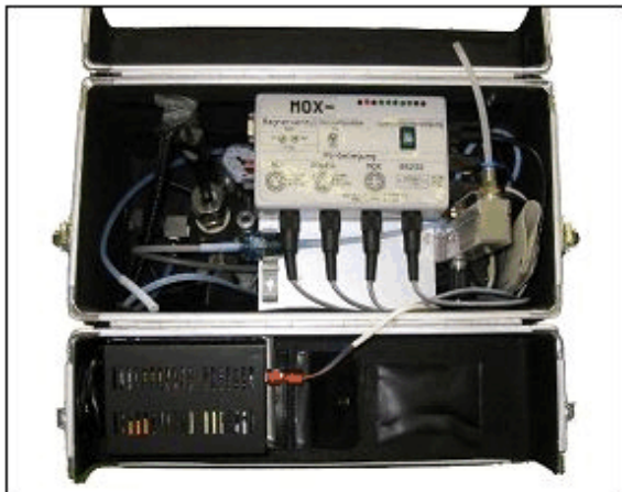
Abb. 9: Metalloxid-Sensorsystem VEGAS (links: Sensorkoffer, rechts: Feldeinsatz)
