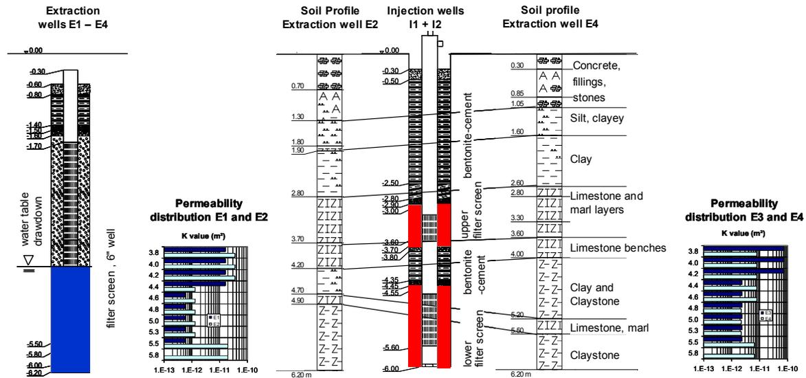
**FIGURE 3. Hydrogeological situation and filter sections of the wells.**
