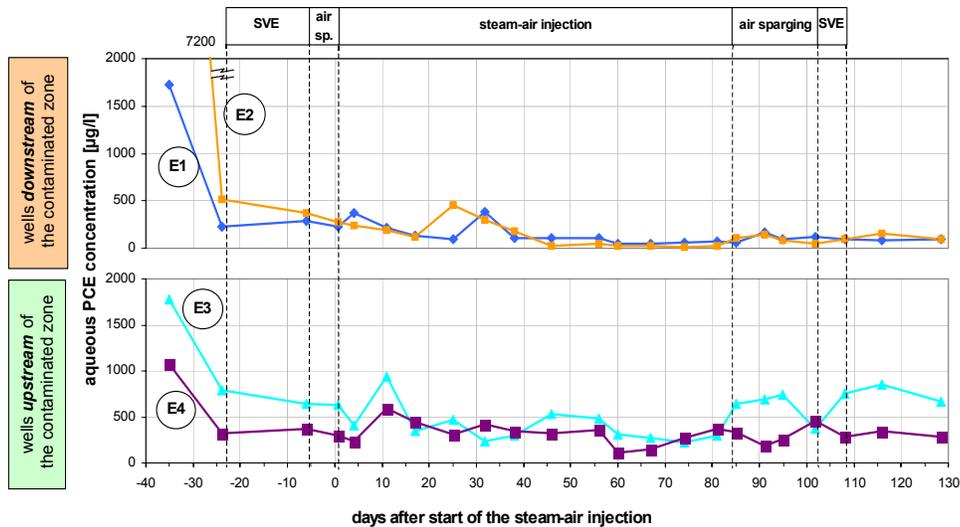
**FIGURE 6. PCE concentrations in the removed groundwater.**
