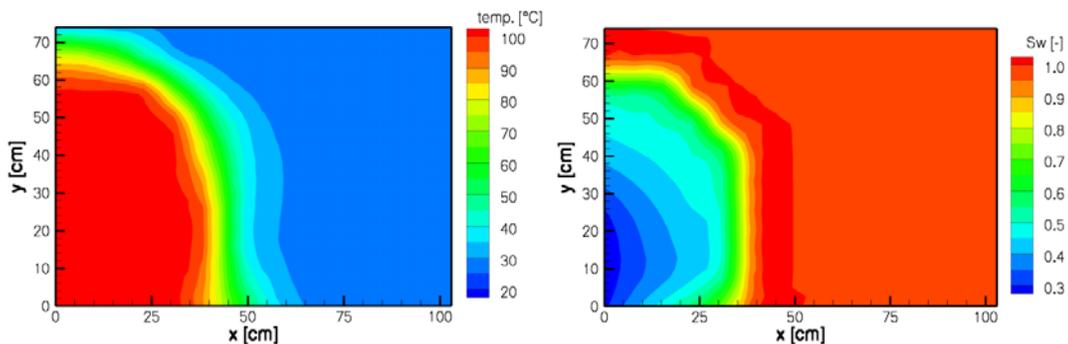
**FIGURE 2. Results from numerical simulations: distribution of temperature (left) and water saturation for a gravity number of 0.8 (right).**
