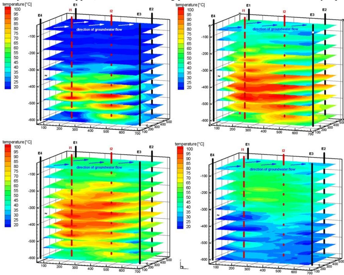
**FIGURE 7. Spatial temperature distribution at 5, 40 (top), 65 and 90 (bottom) days after starting the steam-air injection (lengths indicated in cm).**
