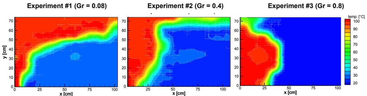
**FIGURE 1. Heat front propagation in a 2-D setup during steam injection into saturated porous media; three experiments with different Gravity number  $Gr$ .**
