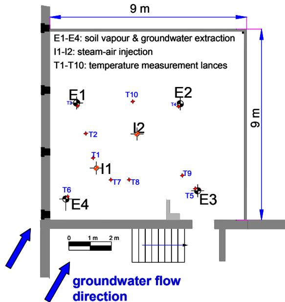
**FIGURE 4. Plan view of the site: extraction wells E1 to E4, while I1 and I2 serve as injection wells for steam-air; T1 to T10 are positions of thermocouple bundles.**
