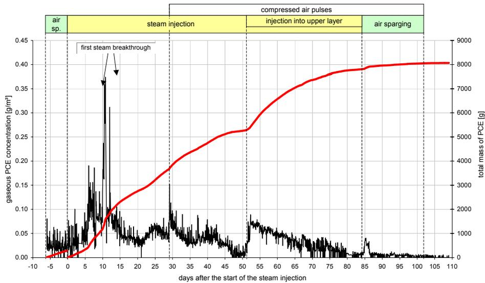
**FIGURE 5. Gaseous PCE concentrations and total mass of PCE removed via SVE.**
