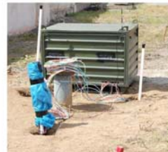
Figure 6. Heads of monitoring arrays for in situ measurement (on Spöckchemie 1 pilot site) connected to measuring hardware in protective box (© VEGAS/USTUTT, University of Stuttgart, Germany).
