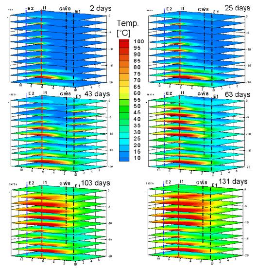
Figure 3: Heat propagation (2 – 131 d of steam injection)
