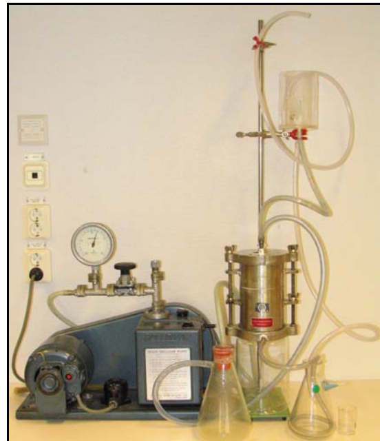
Fig. 6. Permeameter with vacuum device.
