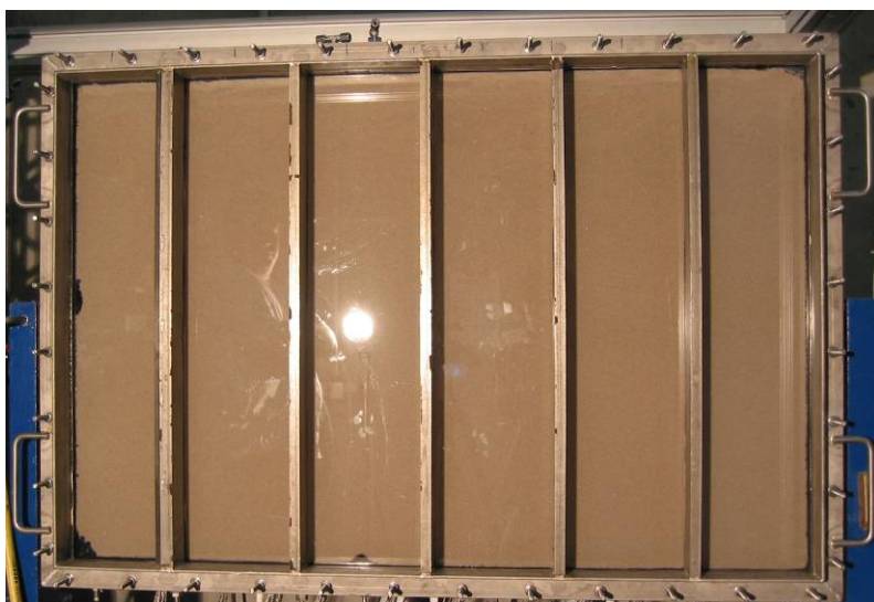
Figure 1: Front side of the 2-D flume.
