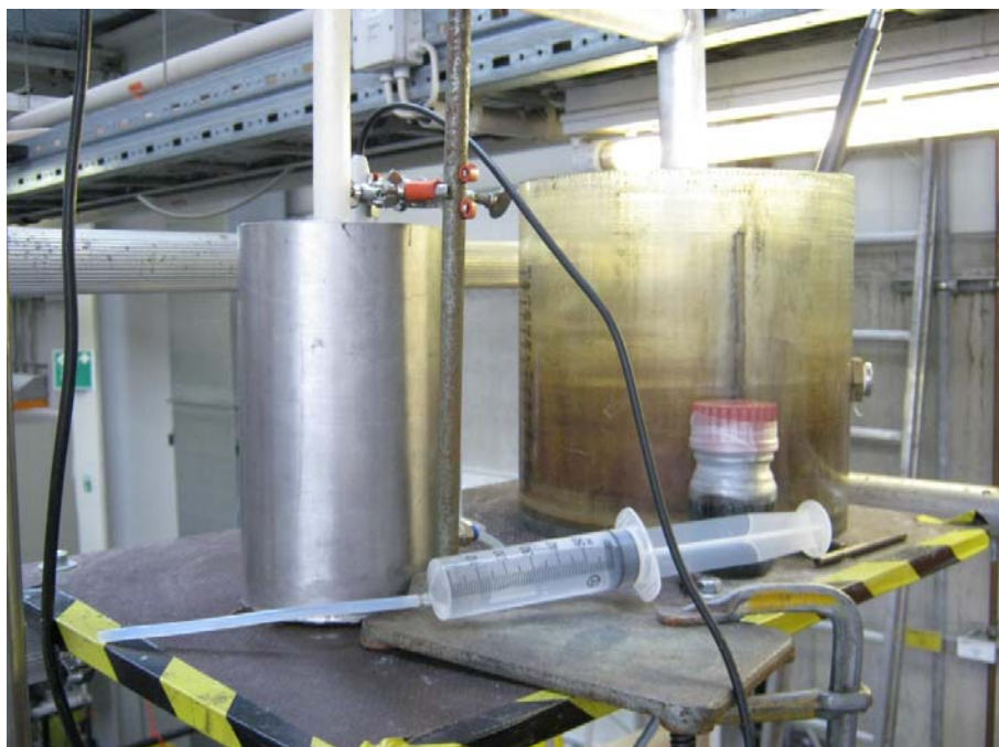
Figure A.3: Measuring the pH of the suspension before adding the iron.
