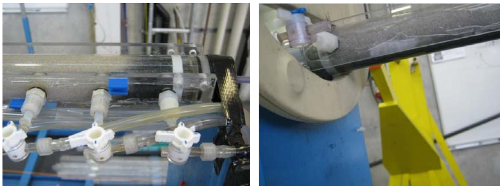
Figure 23: Detail of the measurement ports for the long column (left). The metal detector passing one port (right).
