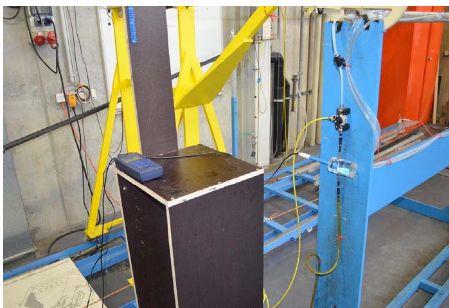
Figure A.4: Continuous pH measurement at the outflow.
