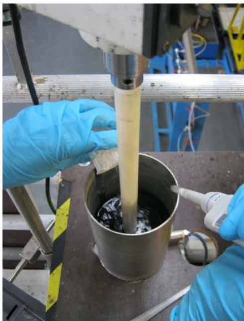
Figure A.1: Sampling for total iron analysis and then pouring the calcium hydroxide.
