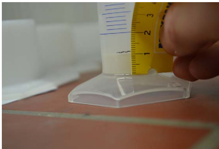
Figure 33: Measurement of the sedimented volume of saturated \text{Ca}(\text{OH})_2 .
