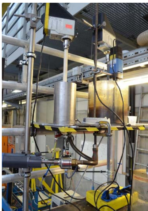
Figure A.2: Injections configuration when iron and calcium hydroxide are injected separately.
