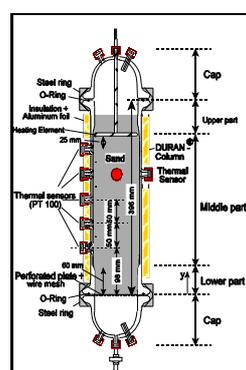
Fig. 1: column setup
