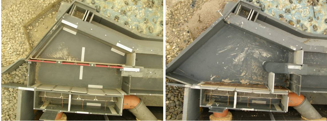
Abb. 10.4: Geometry of the intake house at the beginning (left) and at the end (right) of the investigation
