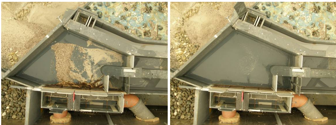
Abb. 10.5: Sediment situation before (left) and after (right) the flushing phase (10 minutes in model)
