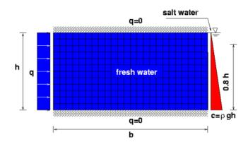
In the figure above, the **mesh and the boundary conditions for the Henry problem** are shown. Initially, the system is filled with fresh water. On the left boundary fresh water influx is prescribed, on the right boundary a hydrostatic pressure distribution.
