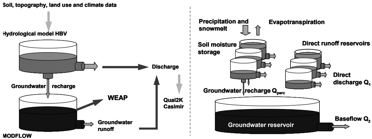
Fig. 7: The groundwater - surface water coupling strategy in RIVERTWIN and the representation of the main processes in the modified HBV model
