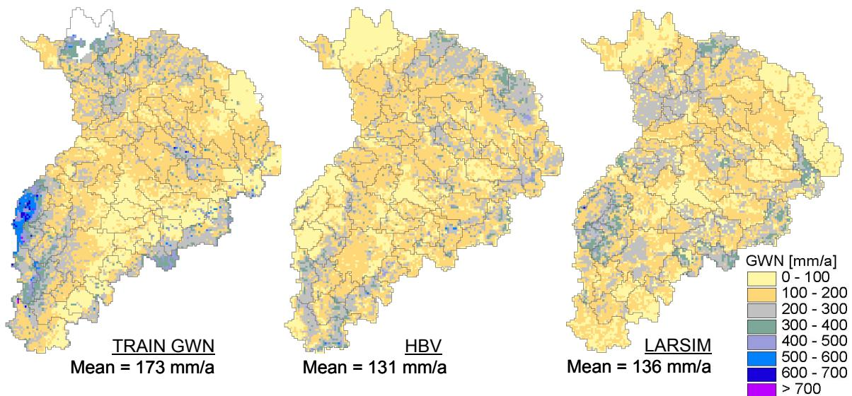
Fig. 8: Spatially distributed recharge averages for the period 1991 to 2001 calculated by three different hydrological models (HBV, LARSIM, TRAIN)
