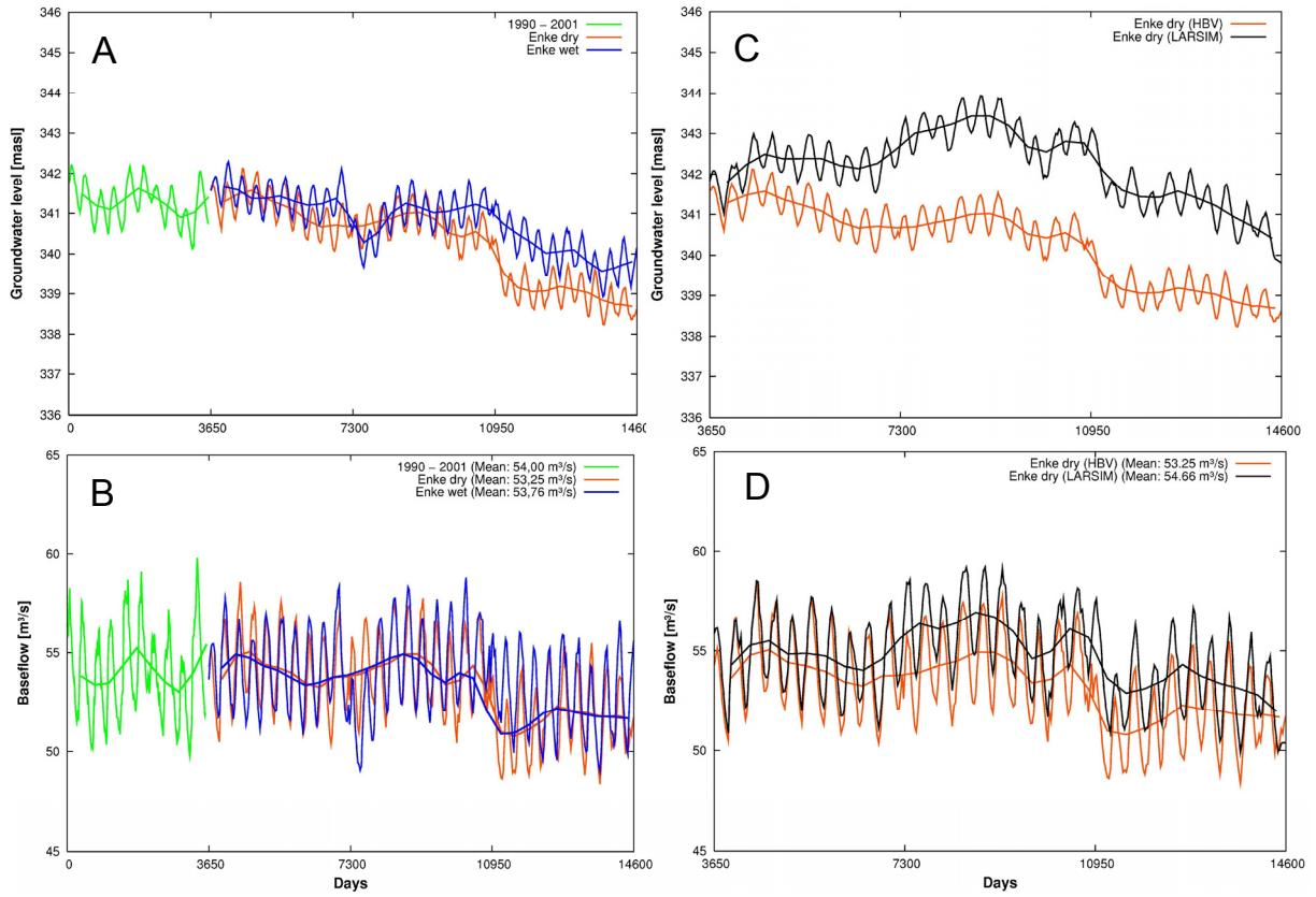
Fig. 9: A and B: groundwater level and baseflow calculated using HBV for two different climate scenarios and the validation period (1991-2000). C and D: groundwater level and baseflow calculated using HBV and LARSIM for the same climate scenario
