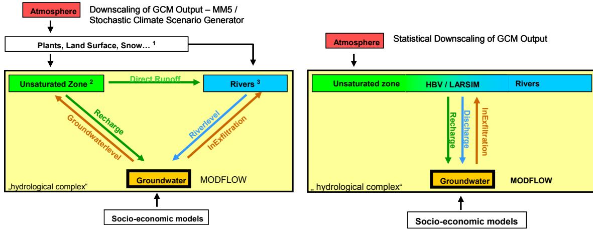
Fig. 6: Coupling (highly schematic) in GLOWA-Danube/DANUBIA (left) and RIVERTWIN / MOSDEW (right)
