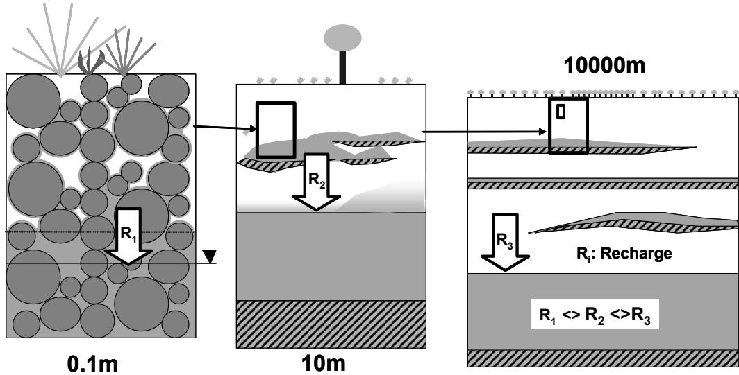
Fig. 5: Groundwater defined at different scales. The relevant definition in groundwater modelling depends highly on the size of the model domain and the discretisation.  $R_1$  to  $R_3$  show the relevant groundwater recharge for each of the relevant aquifers (scales).
