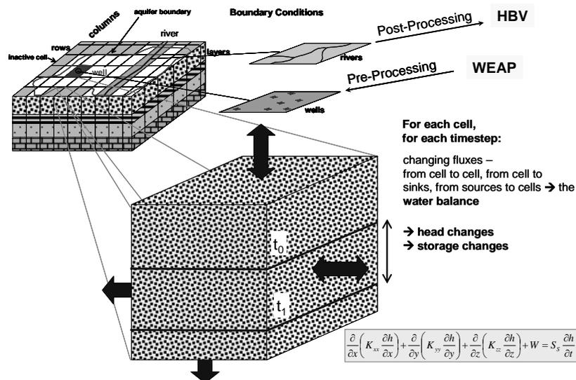
Fig. 4: Principle of the MODFLOW 3D finite difference modelling concept and the provided results.
