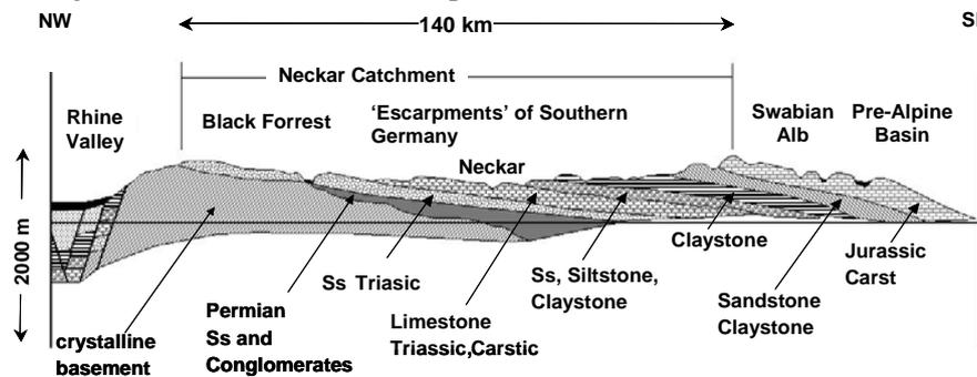
Fig. 2: Geology of the Neckar basin – cross section
