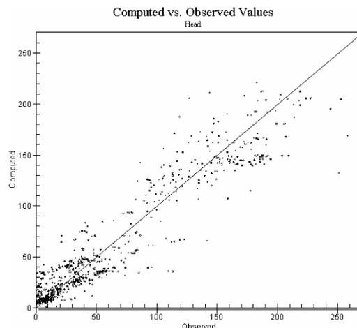
Fig. 6: Results of a steady state calibration of the Ouémé basin groundwater flow model. The diagram combines the results of all four aquifers. All values are in m.a.s.l.
