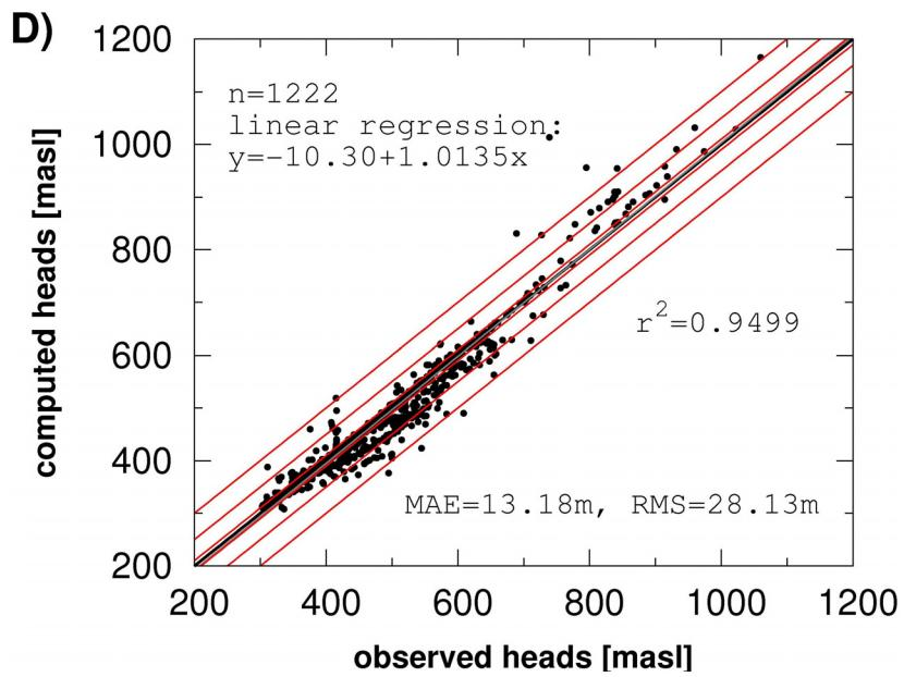
Fig. 4: Stationary model results: observed vs. computed for the Upper Danube catchment model.
