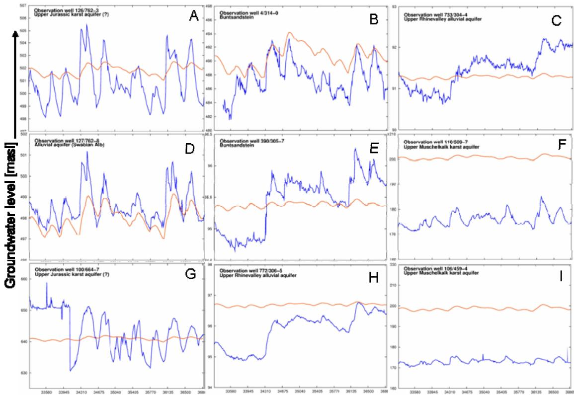
Fig. 6: Transient model results - validation: observed (blue line) vs. computed (red line) groundwater levels for 9 observation wells in different aquifers in the Neckar catchment (1991-2001).
