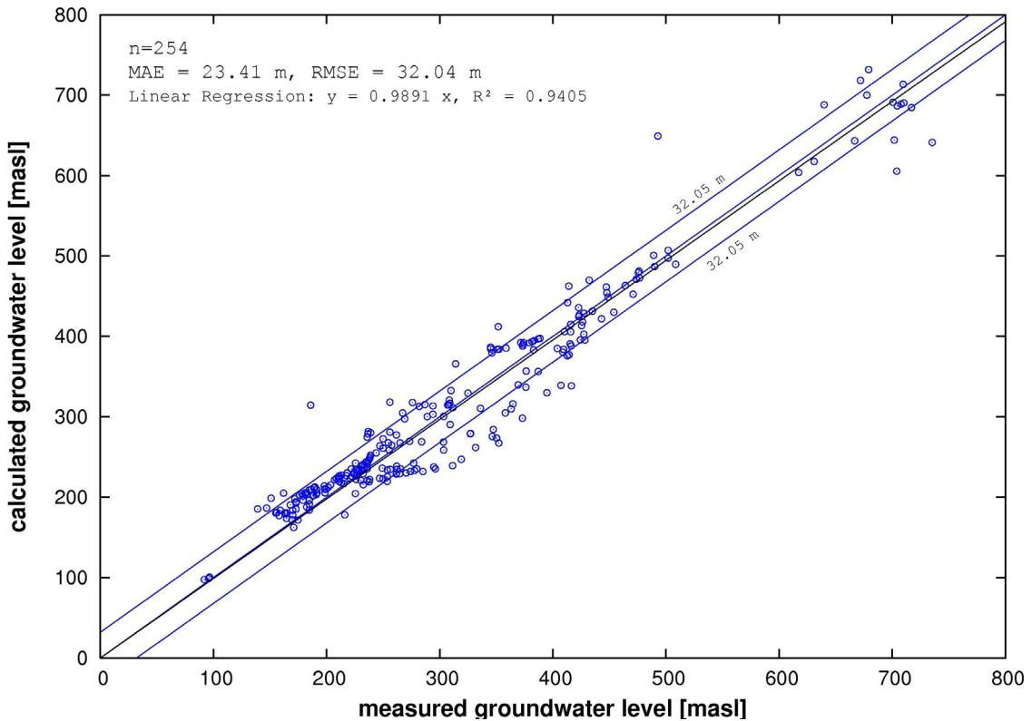
Fig. 5: Stationary model results: observed vs. computed for the Neckar catchment model.
