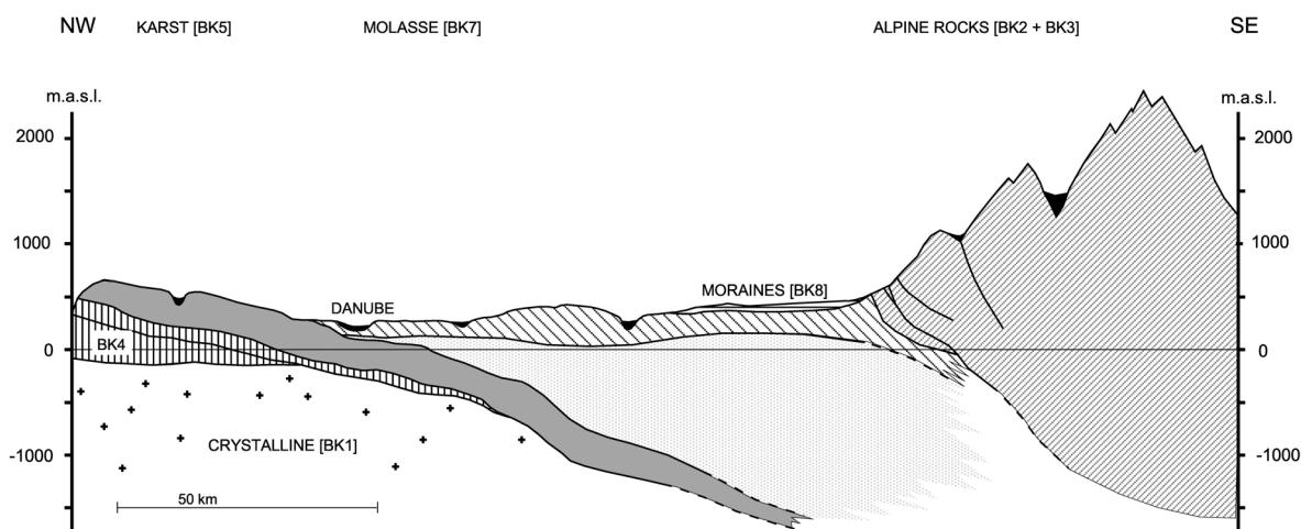
Fig. 2: Geological-hydrogeological cross section of the Upper Danube catchment.
