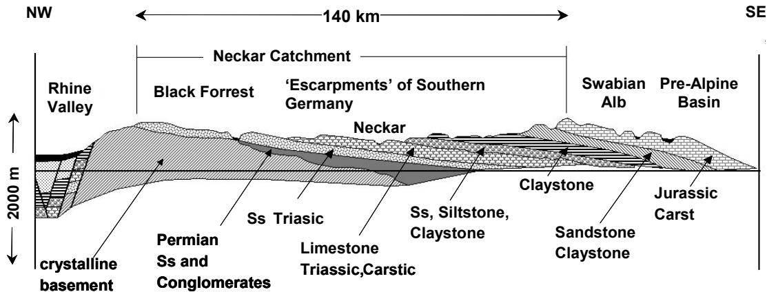
Fig. 3: Geology of the Neckar basin – cross section
