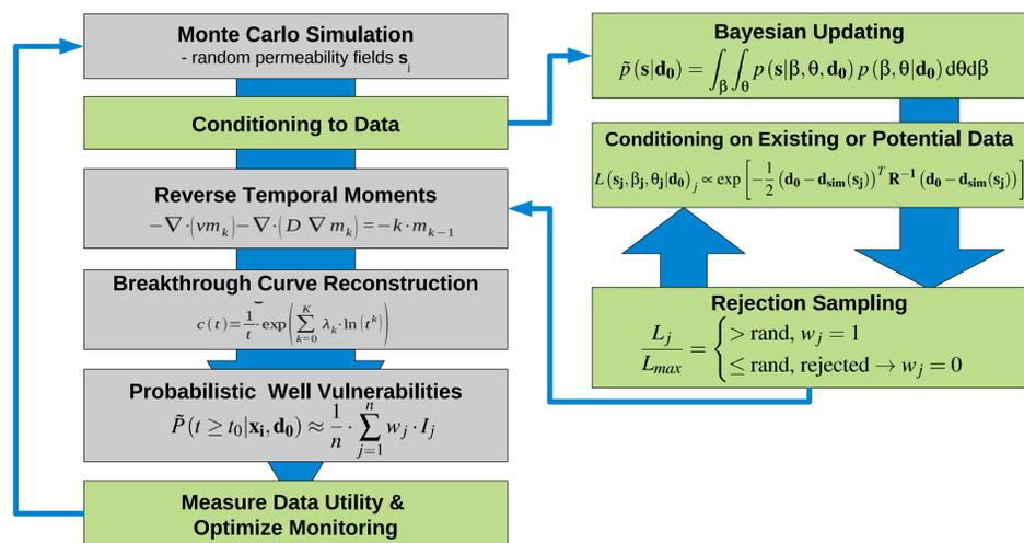
Figure 1: Methodology to determine conditioned probabilistic intrinsic well vulnerability criteria
