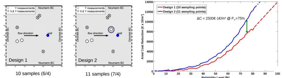
Figure 5: Utility of one additionally planned sampling location to reduce areal costs (Unconditional – Design) through uncertainty reduction ( $U = (A_{R90} - A_{R10}) / A_{R50}$ ) in capture zone delineation.
