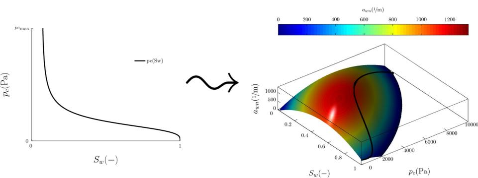
Figure 2: Capillary pressure - saturation relationship (left), capillary pressure - saturation - interfacial area relationship (right)
