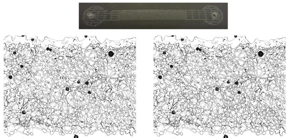
Figure 4: Micro Model (top) and two invasion stages (bottom)
