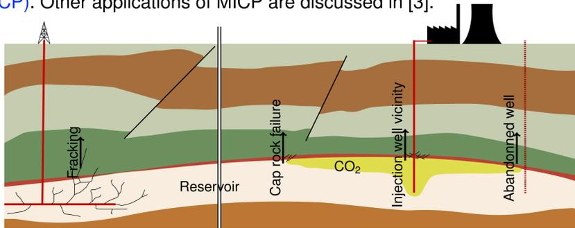
Figure 1: Potential application sites of MICP as a sealing technology in the subsurface.
