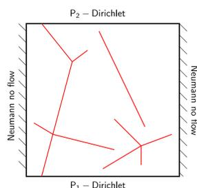
Figure 3: irregular network: domain and boundary conditions
