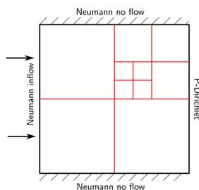
Figure 1: regular network: domain and boundary conditions
