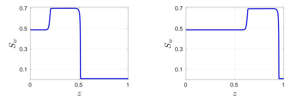
• Case 3:  $S_W^{in} = 0.51$ ,  $c_{im} > c_{dr}$ ,  $t \in \{800 \text{ s}, 1500 \text{ s}\}$ , initial plateau is enlarged
