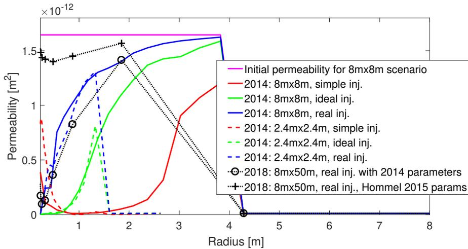
**Fig. 6** Permeability along the radius through the high-permeable layer as predicted by simulations for various grids, domain sizes, and injection strategies. Note that the initial permeability on the left is only shown for the “large” 8 m × 8 m scenario and that for the “small” 2.4 m × 2.4 m scenario, the initial high permeability only extends to a radius of 1.6 m.
