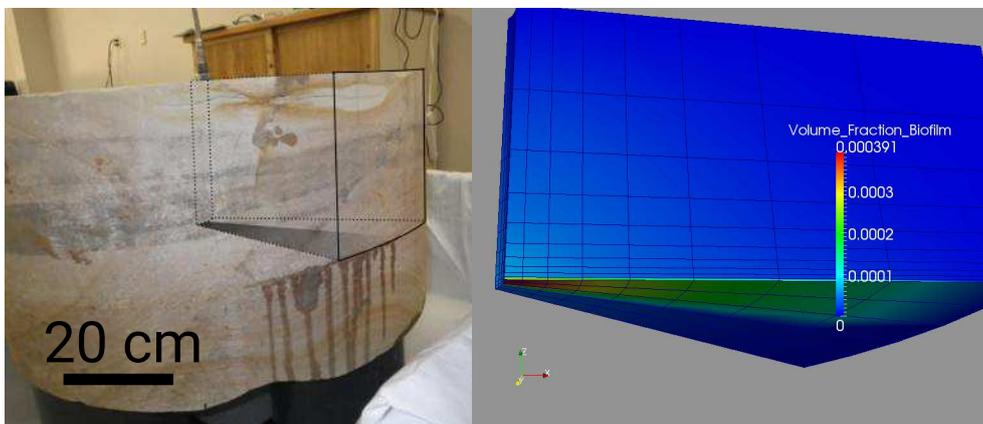
**Fig. 4** MICP modeling of the sandstone-core experiment from Figure 2: (Left) picture of the fractured meso-scale core and a sketch of the simulation domain with the shaded area as the highly permeable layer representing the fracture; the darker areas are indicative of fluids exiting the horizontal fracture. (Right) model prediction of biofilm distribution after 1.16 d of injection. Most of the biofilm is concentrated in the fracture at the front and bottom of the domain.
