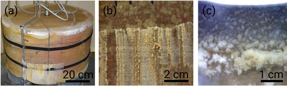
**Fig. 2** Precipitates observed from MICP sealing of a 1 mm fracture (33 cm in length) in a 76.2 cm diameter sandstone core. (a, b) Precipitates formed in the region of the fracture; (c) Precipitates were observed inside the 5.4 cm diameter stainless steel injection tube. These photographs help visualize the nature of the mineral deposits resulting from the application of MICP to seal fractured porous media.
