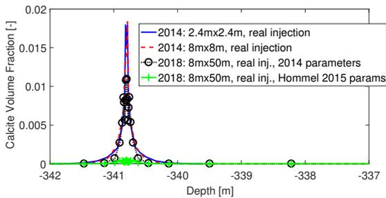
**Fig. 7** Calcite volume fractions at the inner boundary over depth predicted by simulations on various simulation domain sizes. The high-permeable layer into which is injected is situated at 340.8 m below surface.
