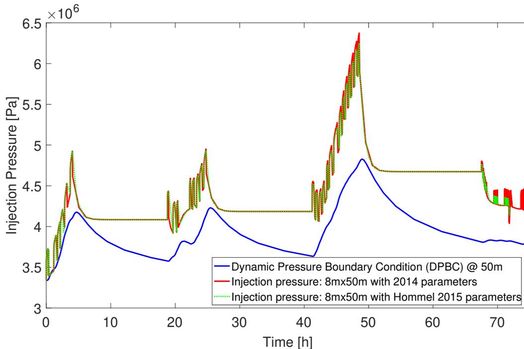
**Fig. 8** Injection pressures as predicted by the model for the “real” injection strategy compared to each other and the dynamic pressure boundary condition pressures set for the 2018 simulations. The dynamic pressure set as Dirichlet boundary condition was determined from simple injection simulations on the same geometry, but a radial extent of 10 km.
