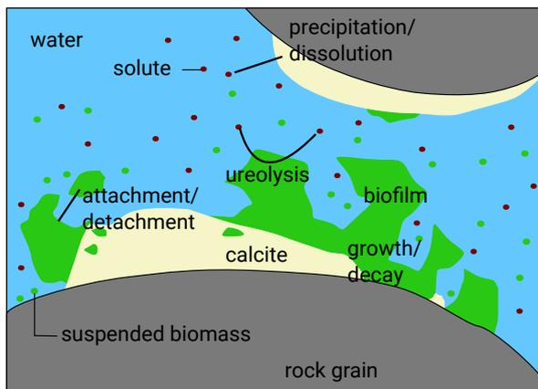
**Fig. 1** Schematic view of relevant processes and phases considered in the conceptual MICP model for the field application scenario, modified from Hommel et al (2015).
