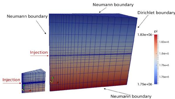
**Fig. 5** Sketch of the grid for the 2.4 m $\times$ 2.4 m and the 8 m $\times$ 8 m and the initial pressure (in Pa) as well as the boundary conditions used for the 2014 simulations.
