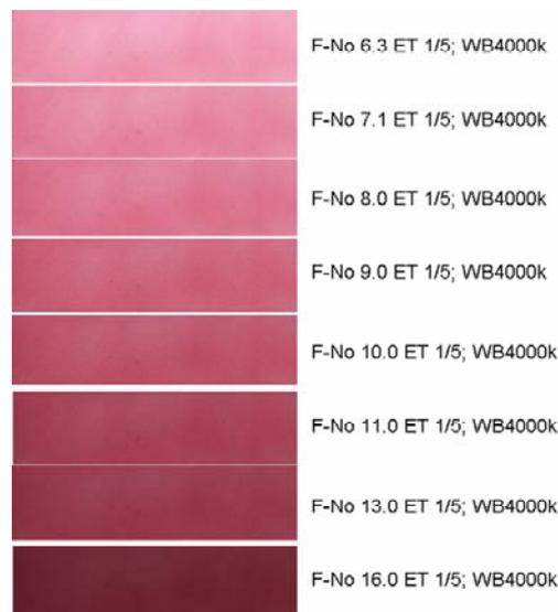
**Figure 15: Variation in the color of the pictures (before being interpreted) by the increase of F-Number for constant exposure time (ET) 1/5 seconds and constant WB4000k. The pictures are taken from the 30% DNAPL saturation experiment.**
