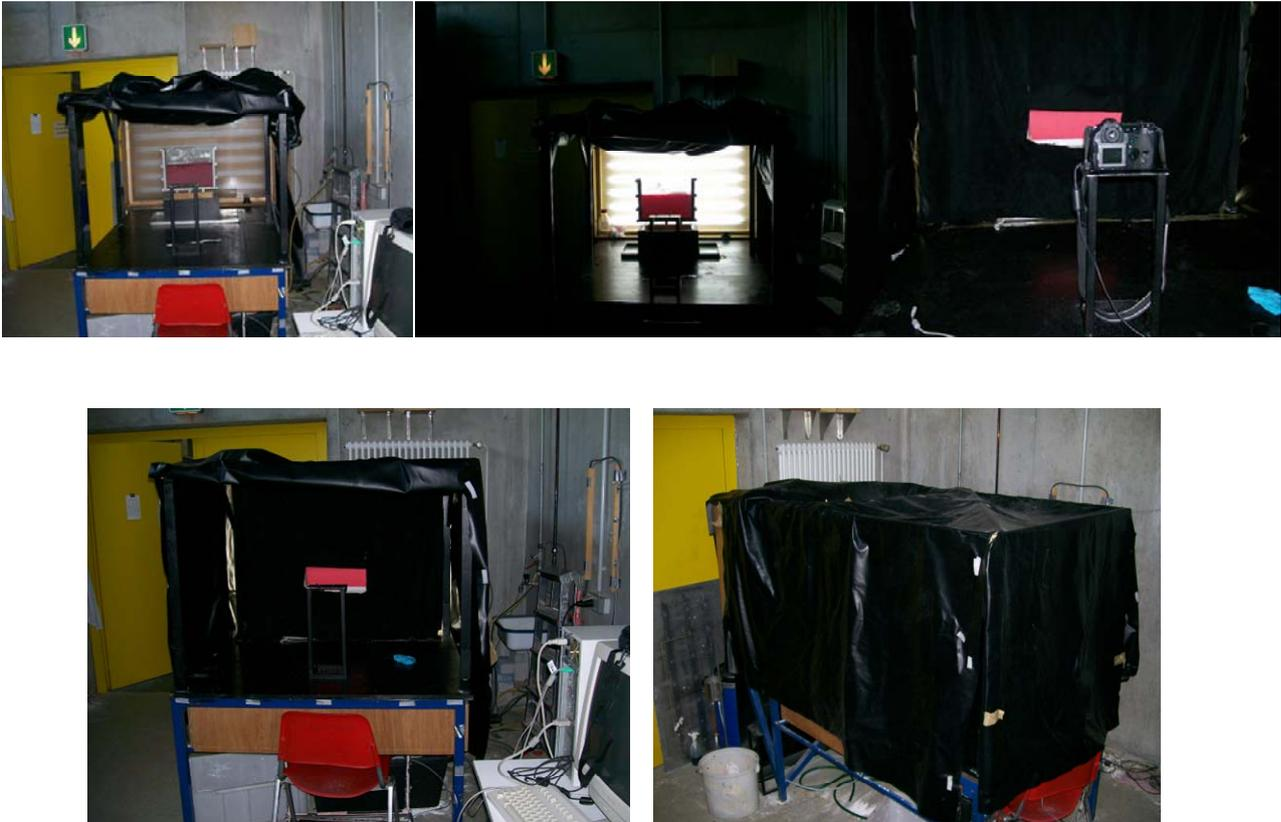
Figure 11: The whole experiment setup: illumination box, slab chamber, camera stand, digital camera, inner and exterior curtains
