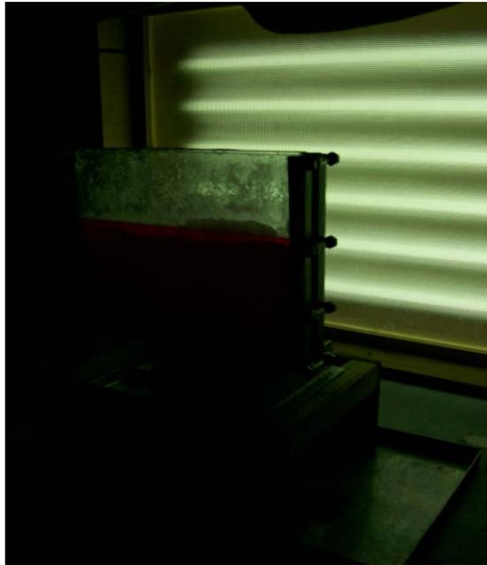
Figure 9: The experimental chamber with the six fluorescent lamps in the background
