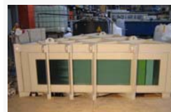
Injection of nano sized zero valent iron (nZVI) in a container with a radial flow field (r = 200 cm, h = 60 cm, Q=1000 l/h, sand: 0.3 – 0.8 mm)
