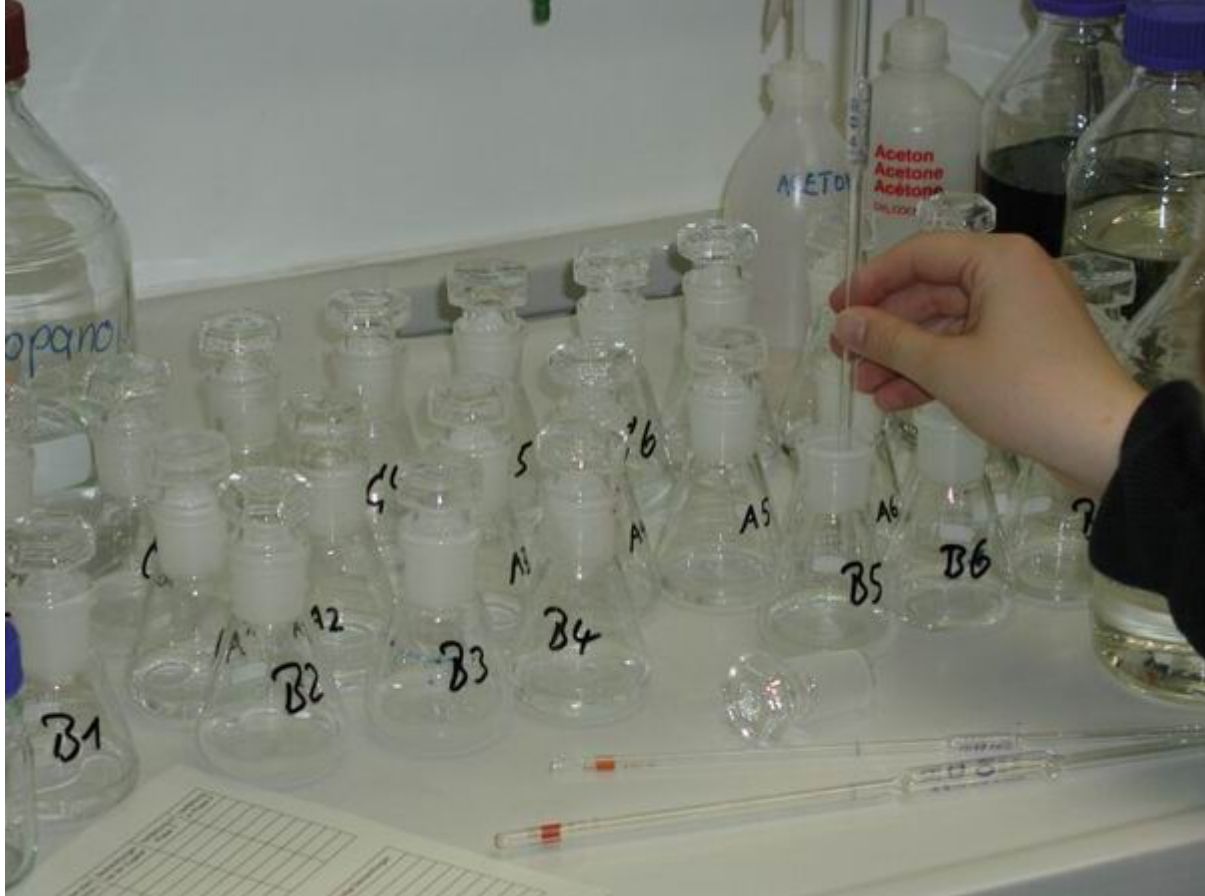
Fig. 2: Preparation of alcohol-water-mixtures to determine the mixing behaviour
