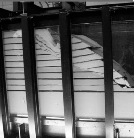
Laboratory experiments were conducted to assess the role of water table position and pore water pressure variation on natural slope stability. Slope failures were found to be preceded by an abrupt decrease in pore water pressure. We suggest that slope stability assessment requires real-time monitoring of pore water pressure variation.
