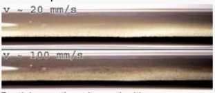
Particles settle at low velocities. (Tube diameter: 5 mm)
