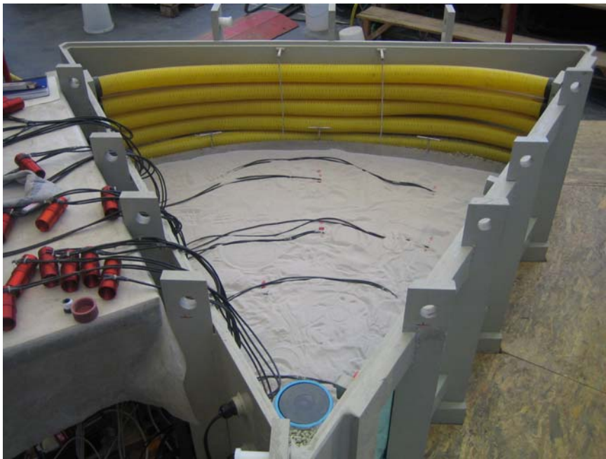
Figure 3: The triangular container during filling with the sensors of the first layer in place.
