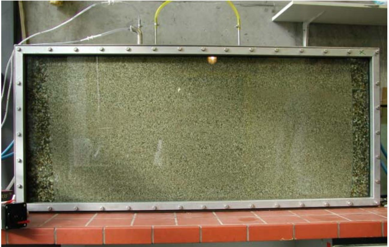
Figure 2: 2-D flume experiment for the visualisation of flow and transport processes using different injection systems
