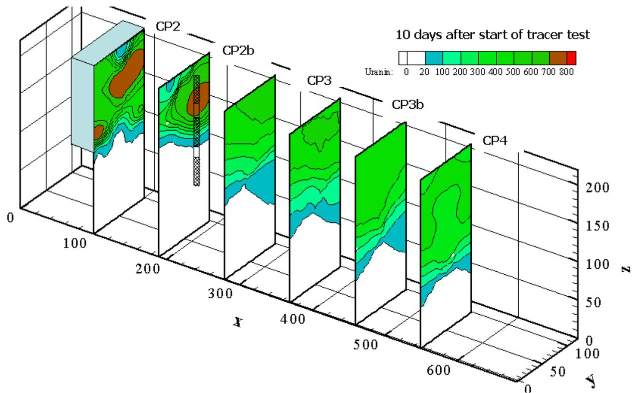
Figure 8: Distribution of the tracer in the Large Flume, 10 days after starting the first tracer test
