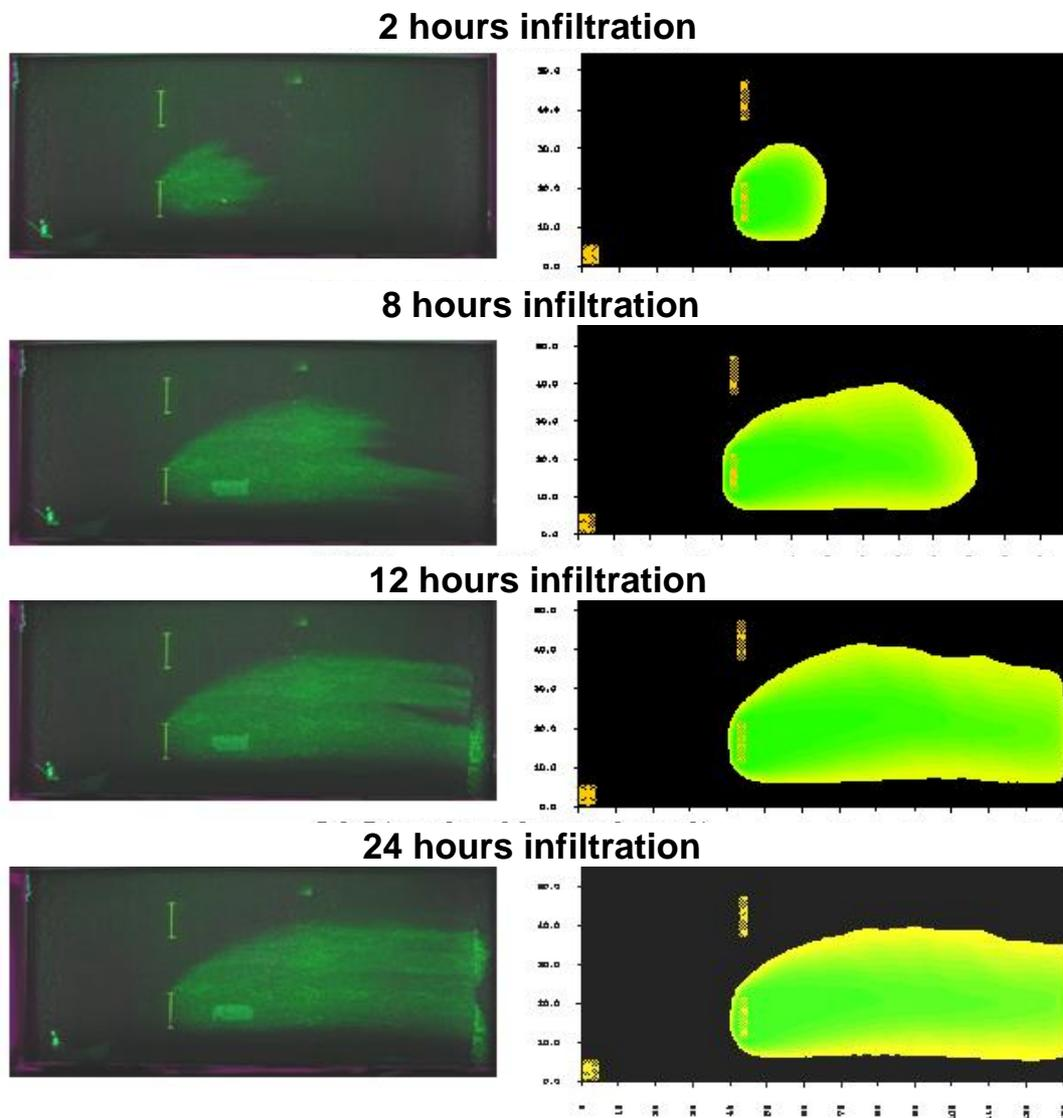
Figure 3: Comparison of experimental (left) and numerical results (right) concerning tracer mixing using GCW
