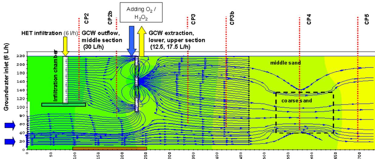
Figure 7: Set up of the Large Flume and the ENA experiment with visualized flow field
