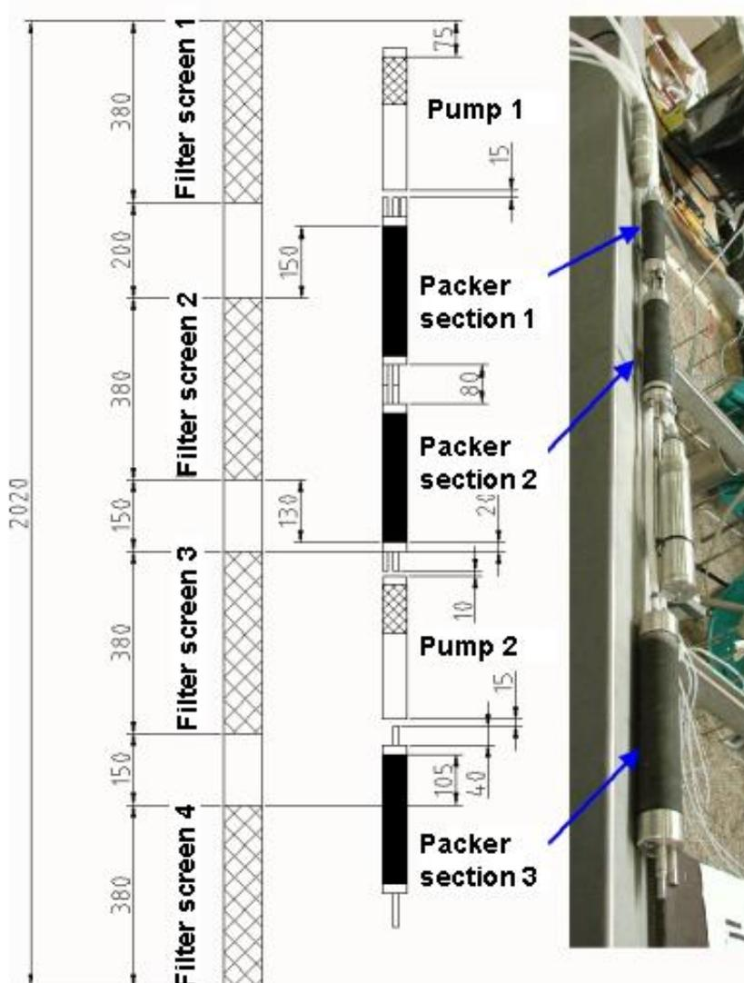
Figure 6: Prototype of the GCW for the application in the Large Flume
