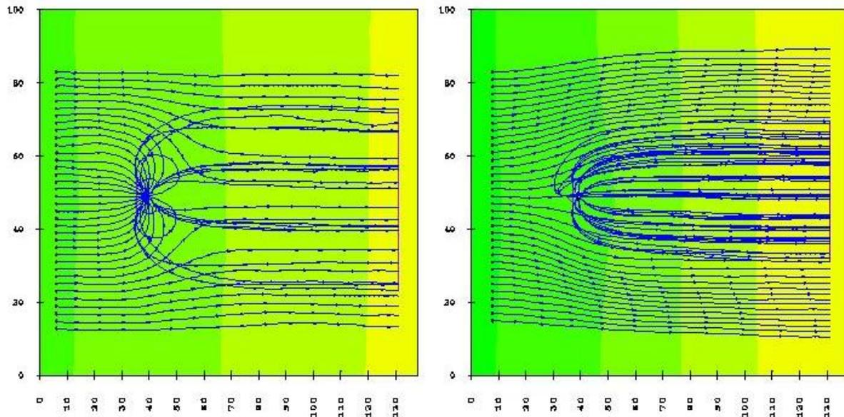
Figure 5: Comparison of flow patterns using GCW (left) and vertical wells (right) for similar infiltration rates
