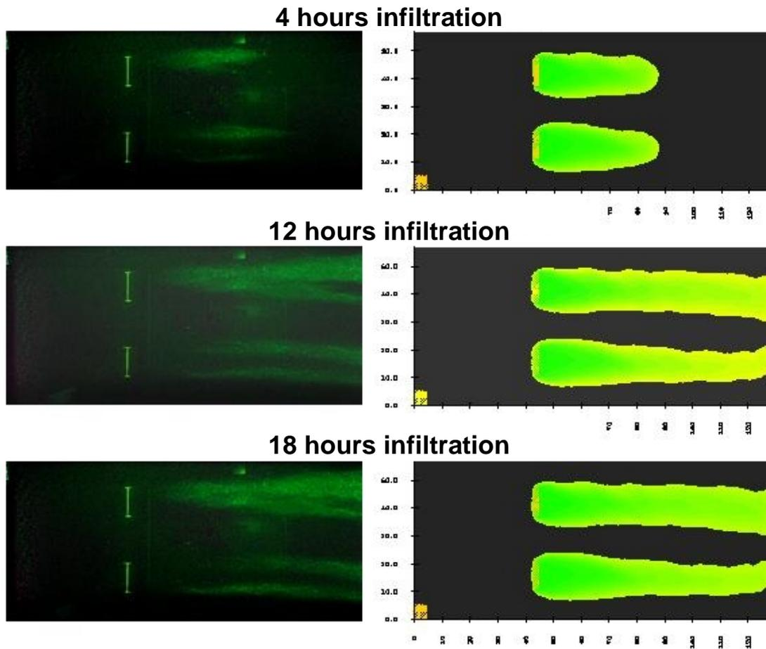
Figure 4: Comparison of experimental results (left) and numerical simulation (right) concerning tracer mixing using MLW
