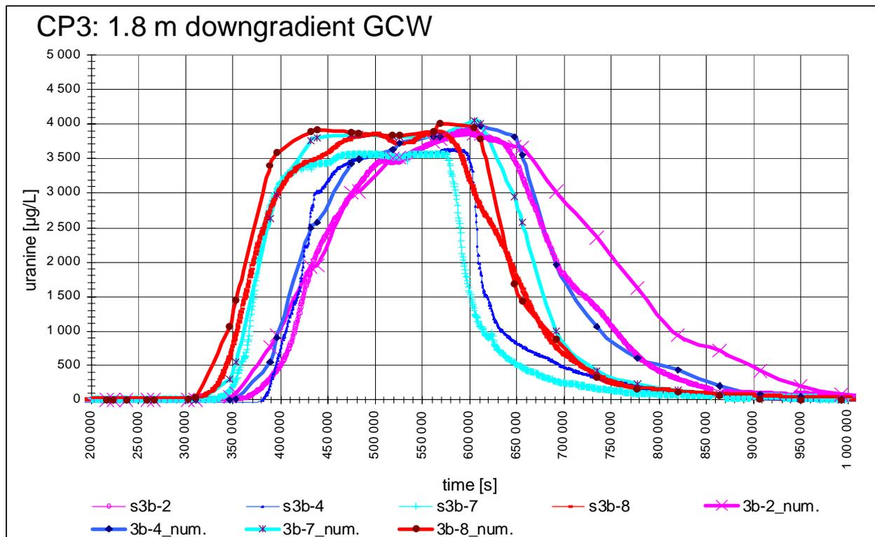
Figure 9: Comparison of the numerically calculated (s3b-2\_num, s3b-4 num, s3b-7 num and s3b-8 num) and experimental tracer breakthrough curves (s3b-2, s3b-4, s3b-7, s3b-8).
