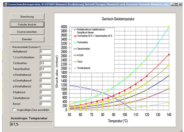
**Azeotropic temperature = co-boiling of steam and CHC depends on pressure**
