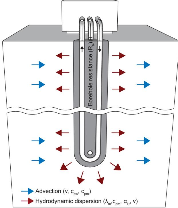
**Figure 1.** Borehole heat exchanger (BHE) during a thermal response test (TRT) with heat transfer processes and parameters accounted for by the moving line source (equation (6)) (thermal borehole resistance  $R_b$ ; Darcy velocity  $v$ ; thermal conductivity of the porous media  $\lambda_m$ ; volumetric heat capacity of the porous media  $c_{pm}$ ; volumetric heat capacity of the groundwater  $c_{pw}$ ; longitudinal and transversal dispersivity  $\alpha_l$  and  $\alpha_t$ ).
