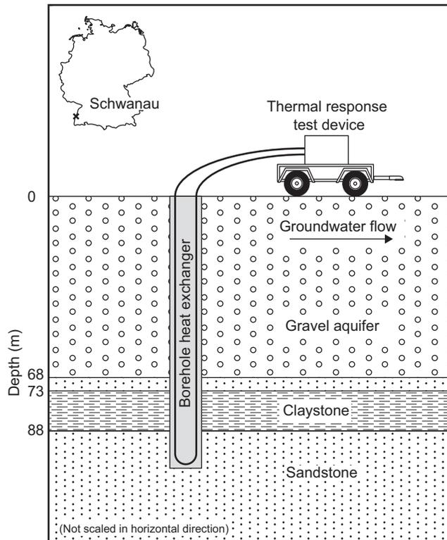
**Figure 8.** Schematic cross section of the studied field experiment in Schwanaun (Germany) showing the layered geological units. The individual depths of the layer boundaries are determined based on borehole cuttings. The depth to water table is only 2 m and is therefore, not explicitly shown.
