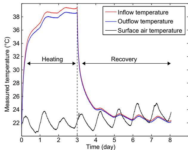
**Figure 7.** Measured temperature development of the heat carrier fluid temperature at the inflow and outflow of the BHE during the TRT experiment at the tank experiment. Additionally, the air temperature in 0.1 m above the surface is shown.
