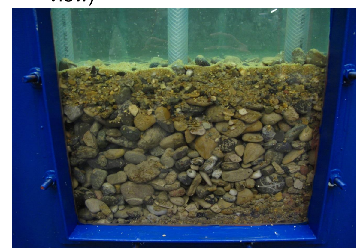
Fig. 5: Introduced coarse cobble layer with 5 cm layer of coarse and fine material on top. (lateral view)
