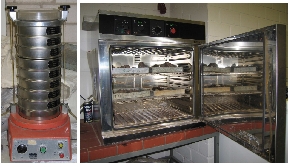
Figure 5.2: Set of sieves mounted on a shaker (left), Drying oven (right)
