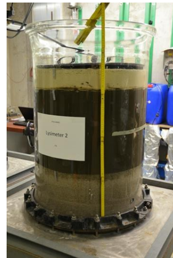
Figure 2: Example of experimental setup (lysimeter)
